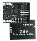
Thank you for purchasing the X89 Brushless Mafia ESC. This ESC has been specifically designed and programmed for general Road Racing.
